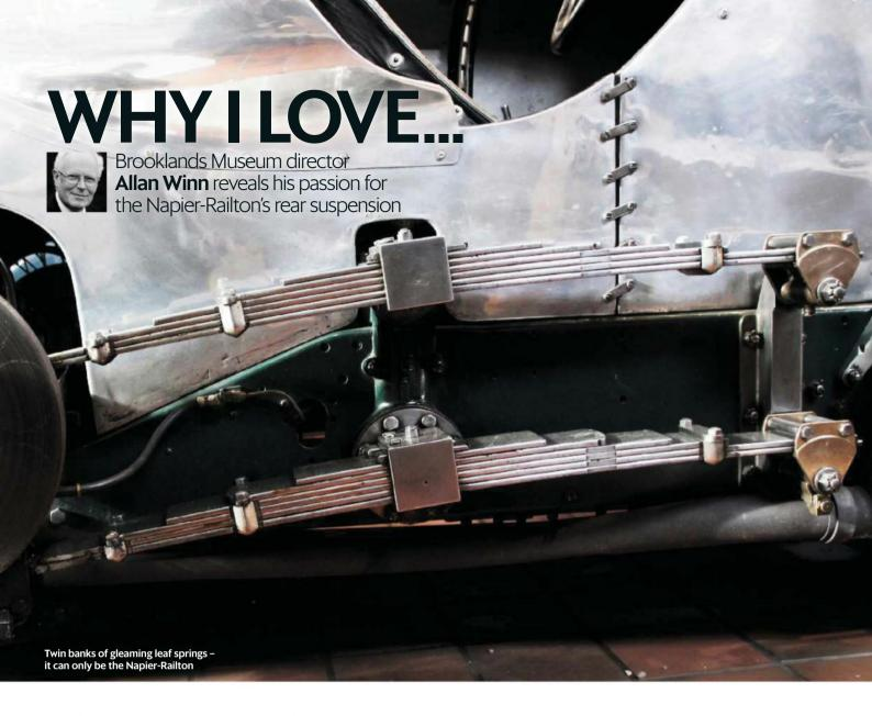
'The set-up controls the suspension movement and power delivery brilliantly. Railton's design for the rear suspension successfully transmits 1300lb ft of torque to the rear wheels without axle tramp'
